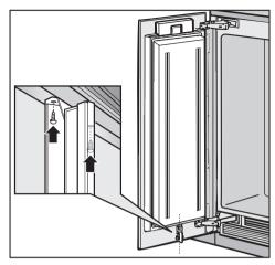
■ Screw the air separator into the middle of the inside of the furniture front, as shown.
